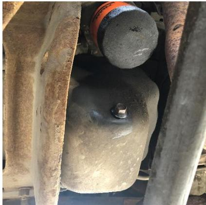
Pictured on the left is a typical front engine, rear wheel drive vehicle. On the right is a front engine, front wheel drive vehicle. Because of the tight space in front wheel drive cars it is good to keep in mind what side of the vehicle the motor is on in comparison to the transmission. It is a good idea to verify this so that you don't accidentally remove the wrong drain plug and empty your transmission of its fluid!
