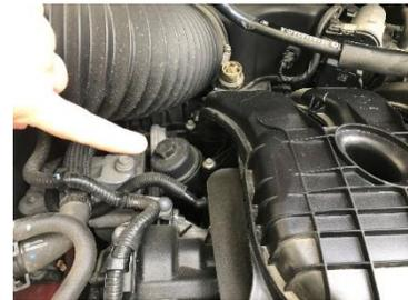
replaces the one on the cap. Have a plastic bag handy to catch the filter when it comes out, so as to not drizzle oil all over your motor. Install the new filter in the same manor in which the old one came out. There is no need to add oil
